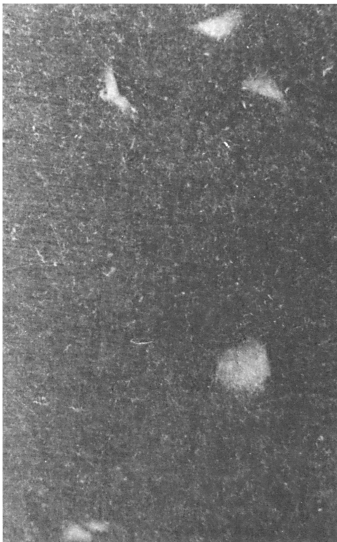
Fig. 3. Optical micrograph of vapor phase-treated sample (1% stearic acid), magnification \times 60 .
