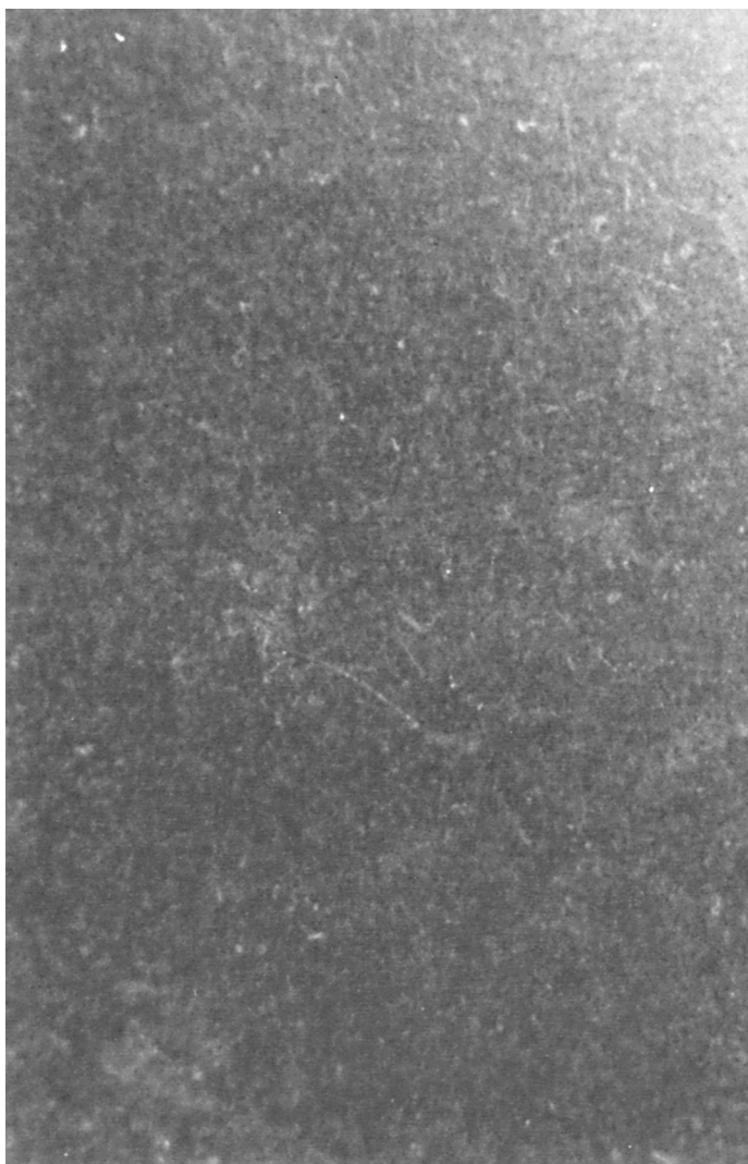
Fig. 5. Optical micrograph of vapor phase-treated sample (3% stearic acid), magnification \times 60 .
